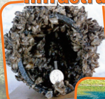
Quagga mussel growth on ABS pipe from Lake Mead, Arizona
